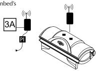
Scenario 3 - T-Max® Manager Series with Wireless combination Wireless can be easily added to an existing salon already utilizing T-Max®. Connect one AP-900 (with Power Injector) to the Manager and one AP-900 to each wireless ready tanning
