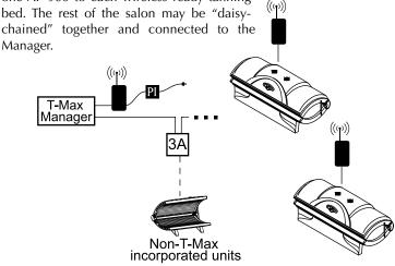
Scenario 4 - T-Max® Manager Series with Wireless combination 2 Connect one AP-900 (with Power Injector) to the Manager and one AP-900 to a wireless ready tanning bed. The rest of the salon may be "daisy-chained" together and connected to the wireless equipped tanning bed, eliminating the need to wire the Manager to the tanning beds.
